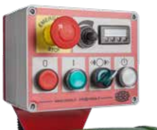
Inverter board: real speed in shown on display.
